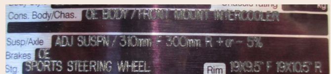
Detail of fake LVV plate showing poorly spaced text and the inch symbol (“).
