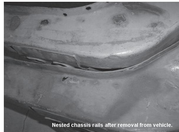
Nested chassis rails after removal from vehicle.
