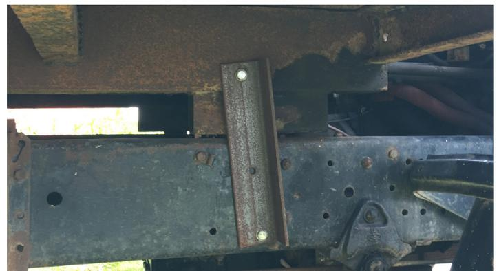
This is not the way to securely mount a deck to a chassis.
