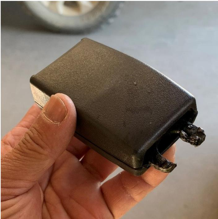
An example of a tampered seatbelt anchor. **7-5 Seatbelts and seatbelt anchorages** reason for rejection 13(c) says to fail if you see a seatbelt anchorage that is corroded, damaged or shows signs of tampering.
