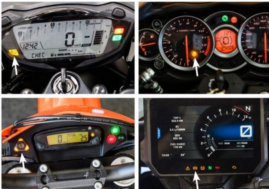
Figure 8-1-1. Examples of ABS warning light fault indication
