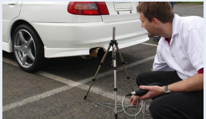
Objective noise tests being carried out
