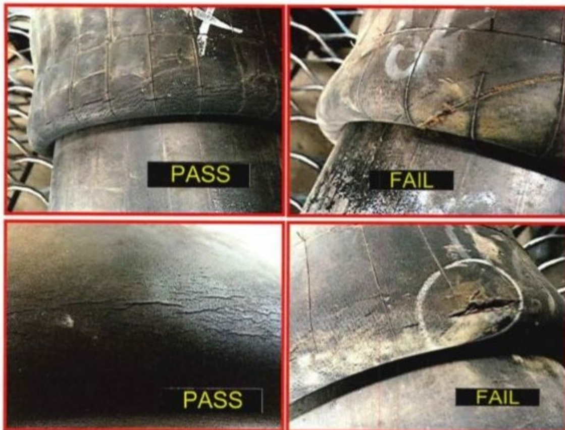
Figure 9-1-2. Sample air bag bellows images
