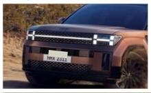
Lights that are made up of several segments (an array), and could include headlights or DRLs, must be treated as 1 unit and the reasons for rejection require 75% of the segments to be working.
