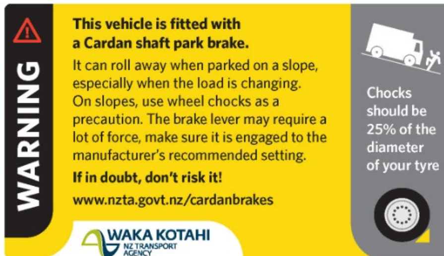
Figure 8-1-6. Cardan shaft park brake warning sticker
