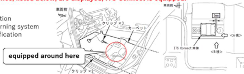
※ Navigation system may be removed but ITS Connect system unit can be left equipped for used vehicles. ITS Connect unit can be found under the floor mat of passenger seat
