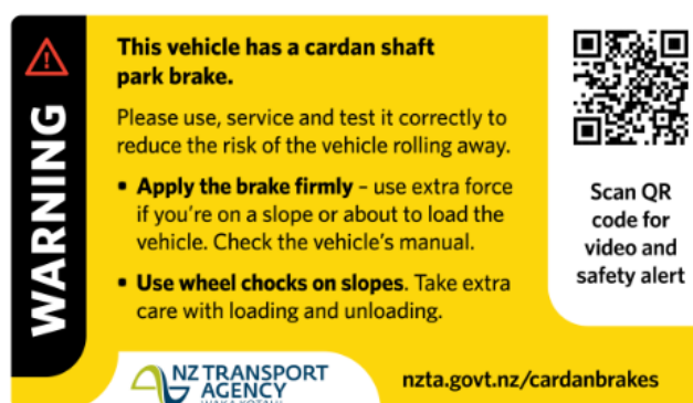
Figure 5-1-1. Cardan shaft park brake warning sticker
