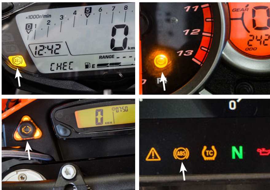
Figure 8-1-1. Examples of ABS warning light fault indication
