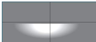
Modern symmetric dipped beam headlamp pattern on light board
