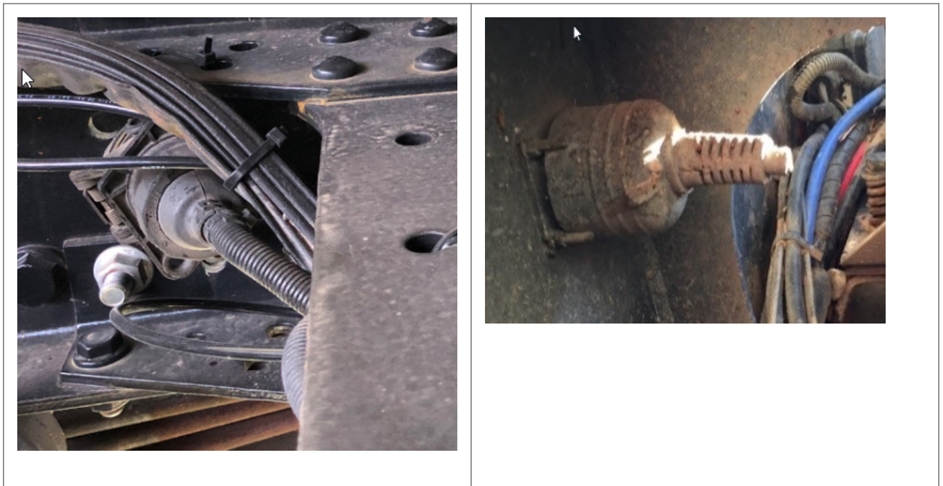
Check wheel sensors and pulse rings (if visible) and for trapped wiring or damaged air lines.
