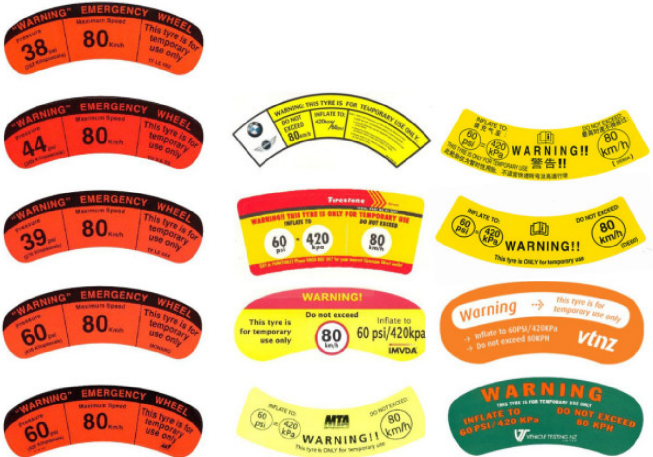
Figure 10-1-3. Common space-saver tyre labels
