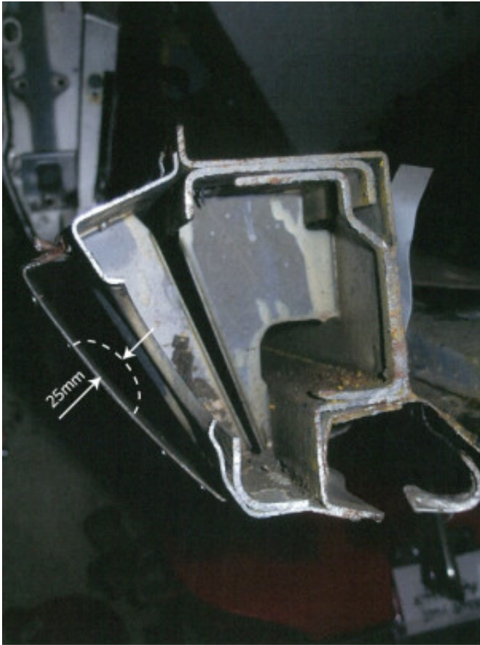
Figure 3-4-1. Outer sills cross section and rocker panels
