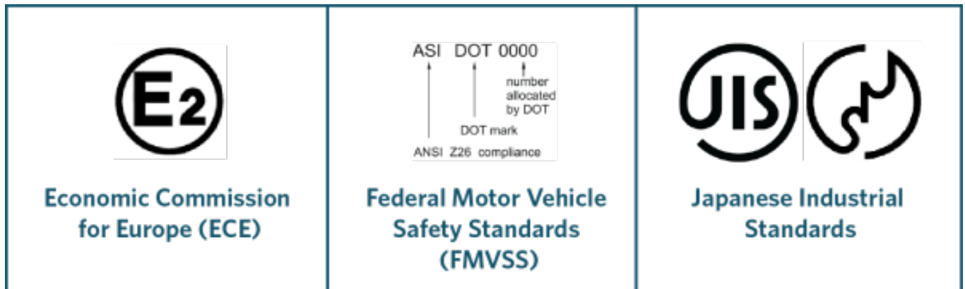
Figure 4-11-1. Approved high-mounted stop lamp standard markings
