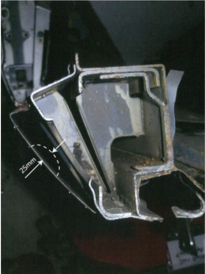
Figure 3-4-1. Outer sills cross section and rocker panels
