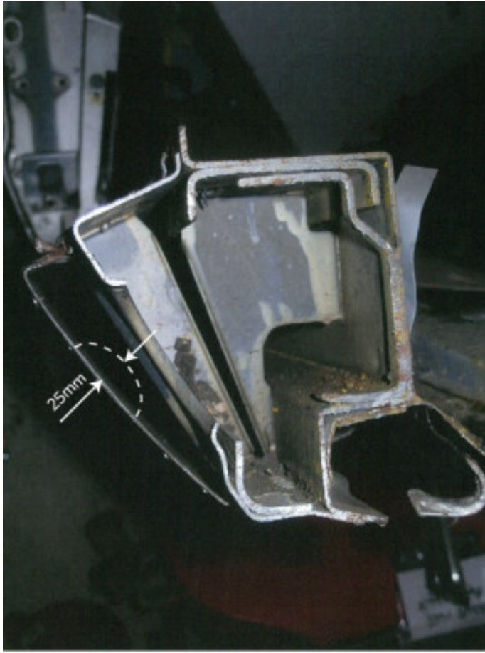
Figure 3-4-1. Outer sills cross section and rocker panels
