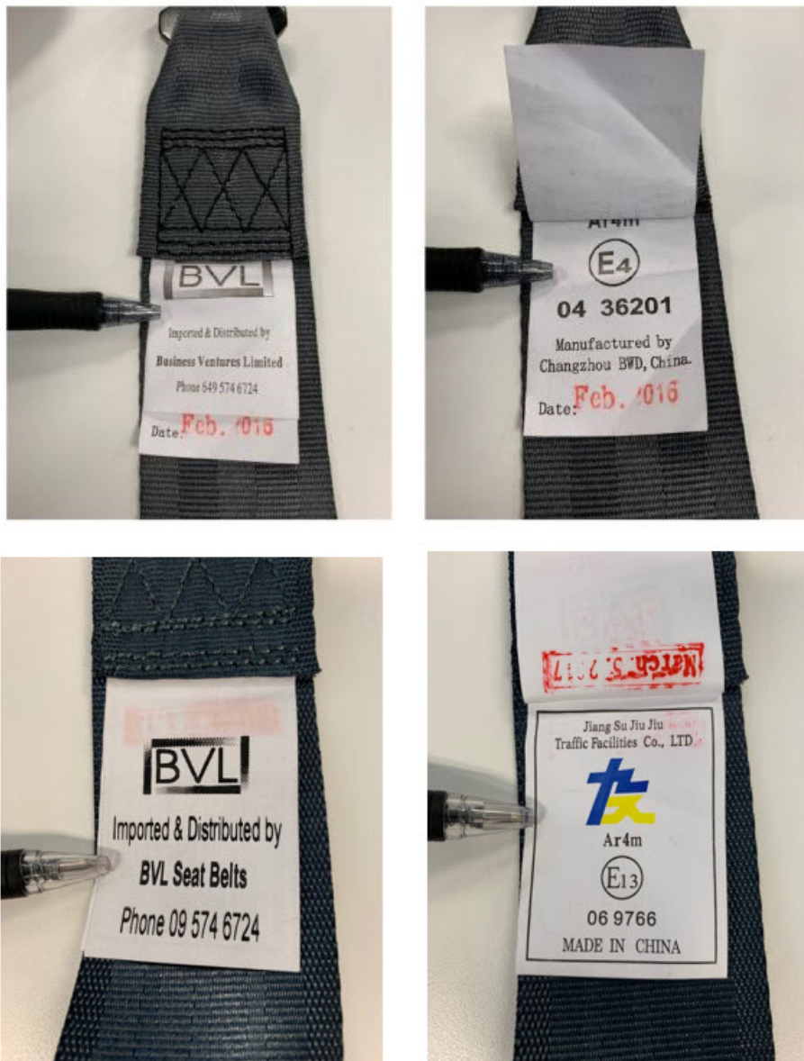
Figure 7-5-2. Identifying seatbelts by BVL (Business Ventures Limited) and manufactured by Changzhou BWD, China or Jiang Su Jiu Jiu Traffic Facilities Co. Ltd.
