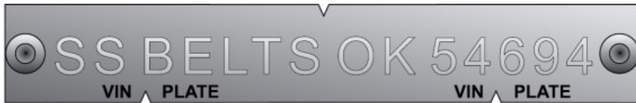
Figure 17-1-1. Example of a plate fitted to a vehicle that may retain a single-sensitive seatbelt
