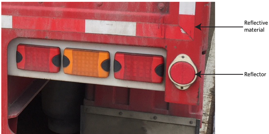
Figure 4-13-3. Examples of ADR, UNECE, and JIS combination lights with built-in reflectors
