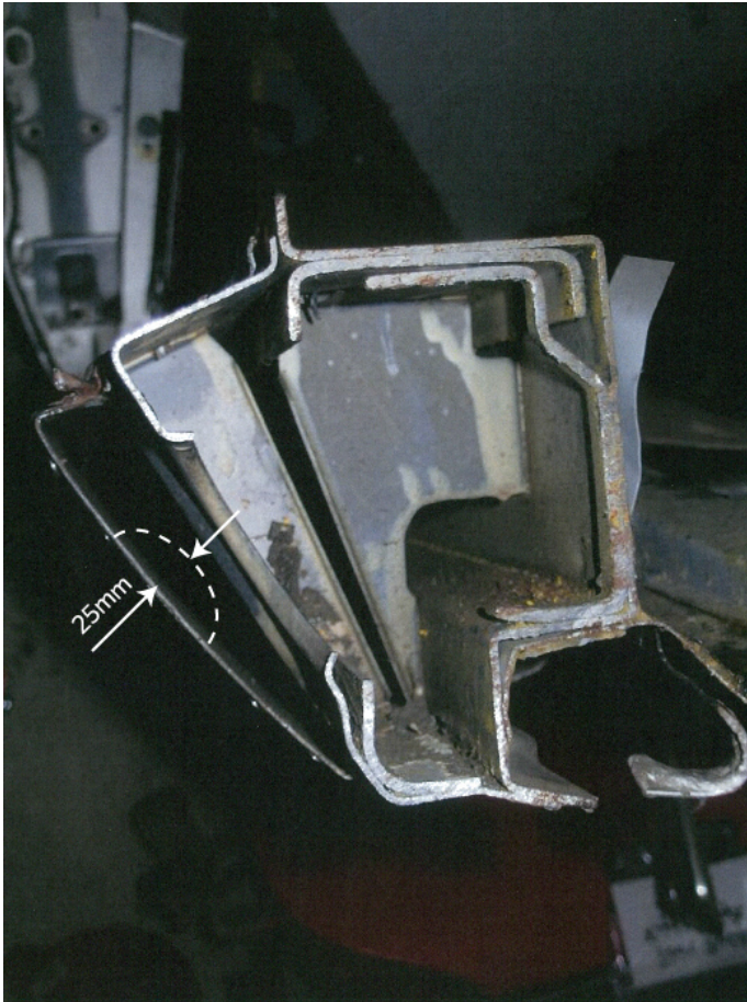
Figure 4-1-1. Outer sills cross section and rocker panels
