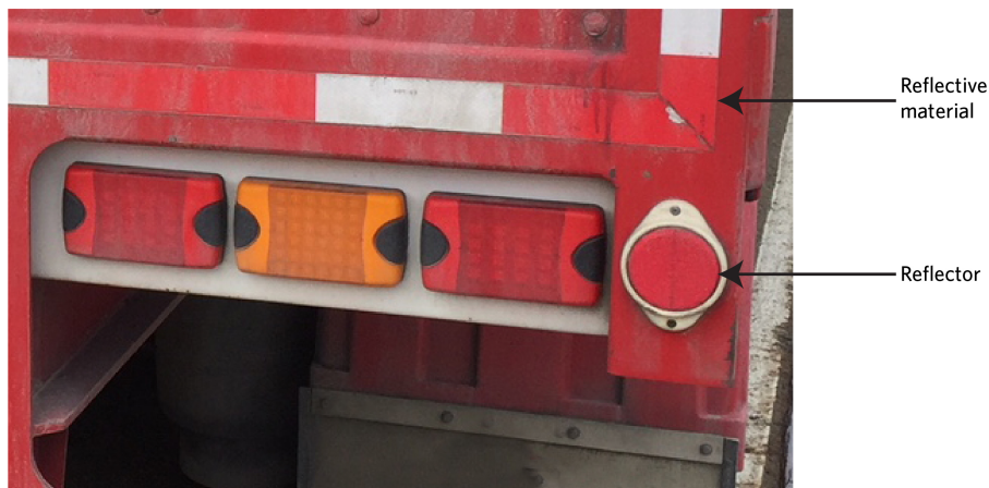
Figure 4-13-2. Reflector vs reflective material
