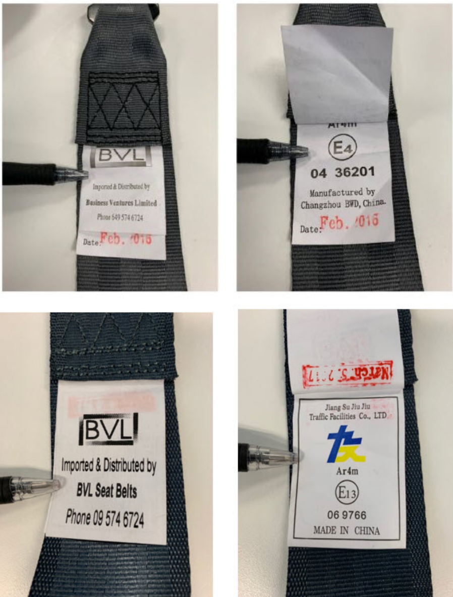
Figure 7-5-1. Identifying seatbelts by BVL (Business Ventures Limited) and manufactured by Changzhou BWD, China or Jiang Su Jiu Jiu Traffic Facilities Co. Ltd.
