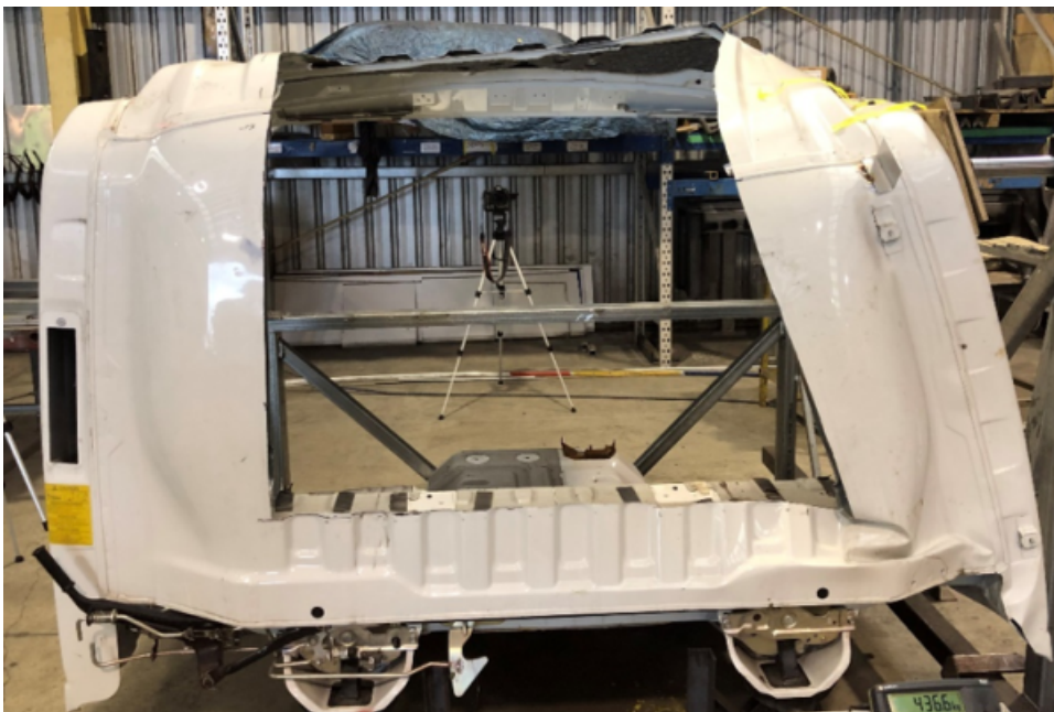
Figure 20-1-4. Modification to the rear wall and roof, Japanese (during testing)
