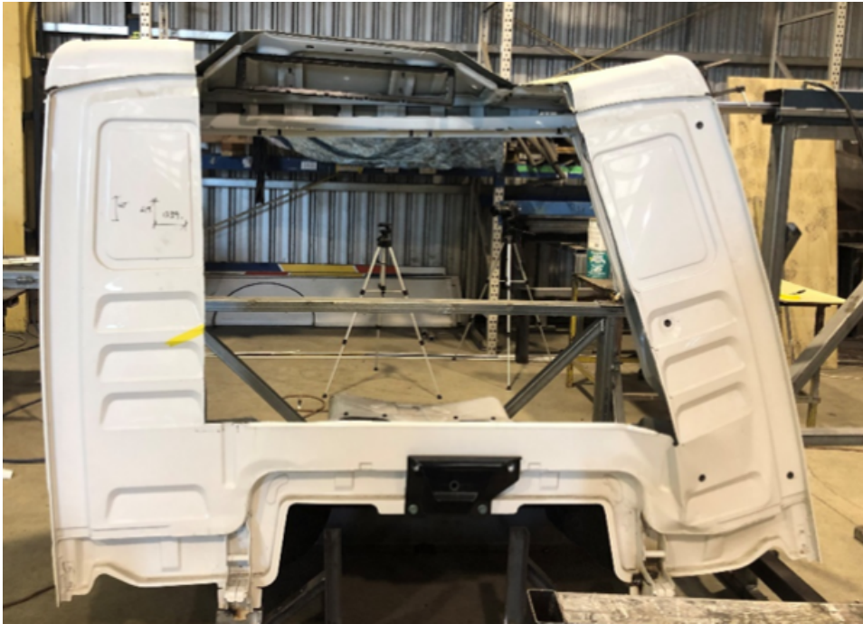
Figure 20-1-5. Modification to the rear wall and roof, European (during testing)
