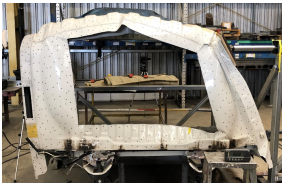
Figure 20-1-2. Modifications to the rear wall only, Japanese (after testing)
