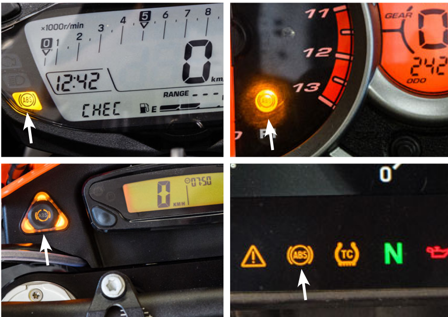
Figure 8-1-1. Examples of ABS warning light fault indication
