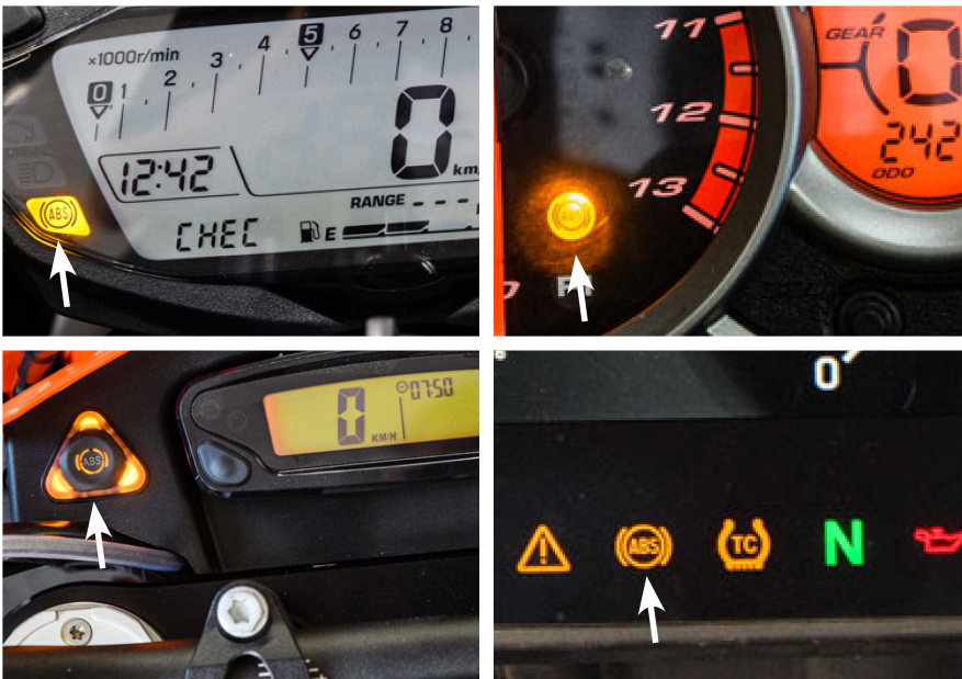
Figure 8-1-1. Examples of ABS warning light fault indication
