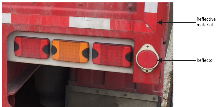
Figure 4-13-1. Reflector vs reflective material
