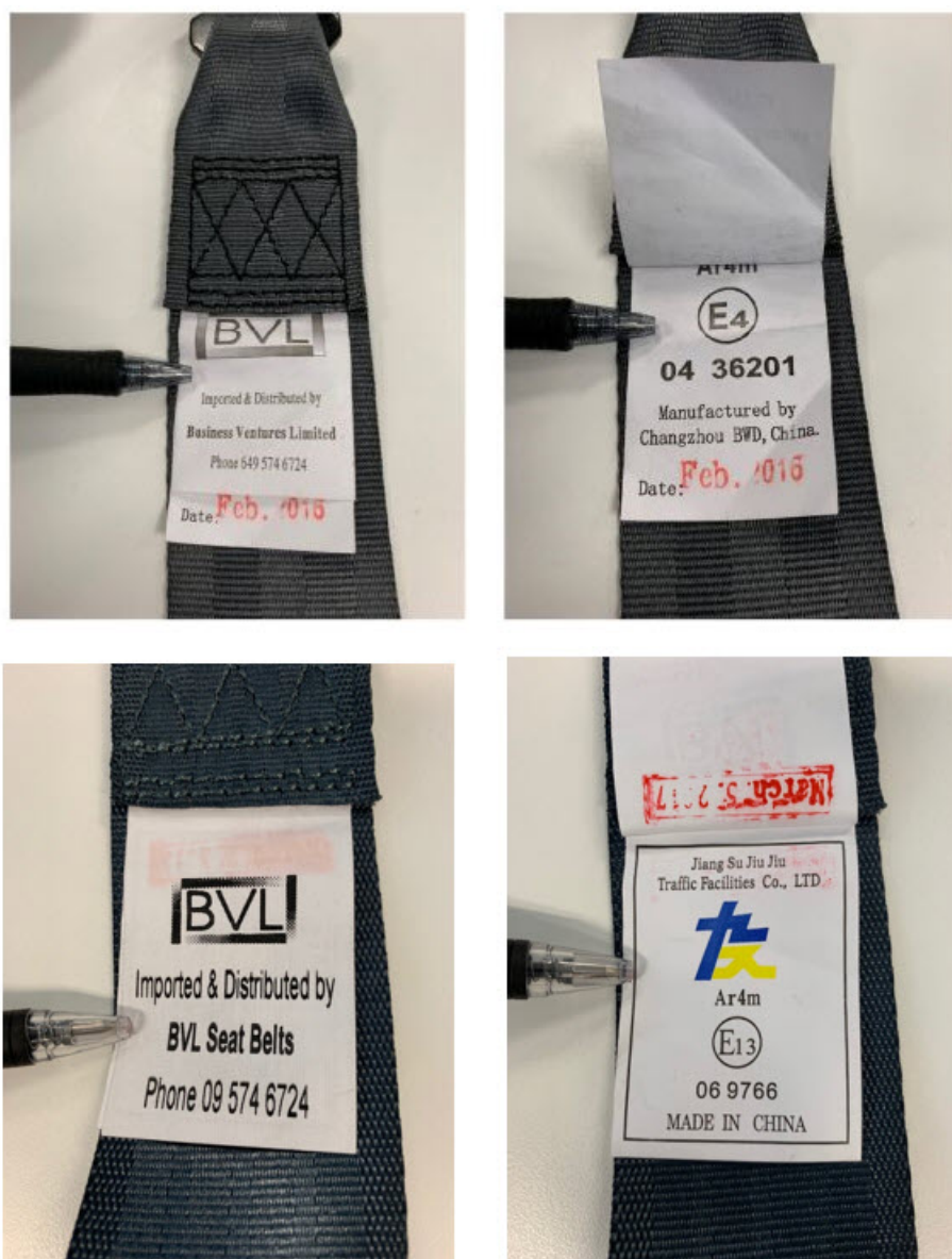
Figure 7-5-1. Identifying seatbelts by BVL (Business Ventures Limited) and manufactured by Changzhou BWD, China or Jiang Su Jiu Jiu Traffic Facilities Co. Ltd.
