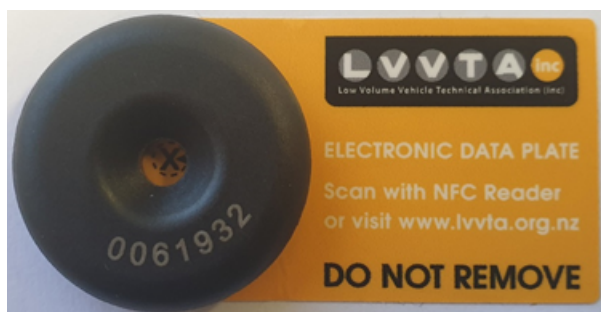
Figure 1-7-1 Sample LVVTA electronic data plate
