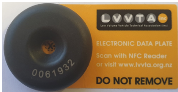
Figure 1-7-1 Sample LVVTA electronic data plate
