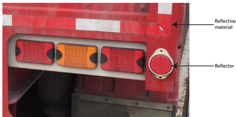
Figure 4-13-1. Reflector vs reflective material
