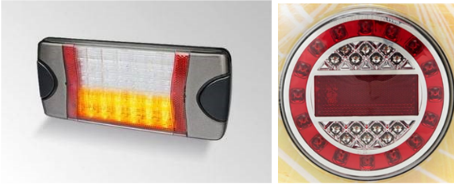
Figure 4-13-4. Examples of single retroreflector
