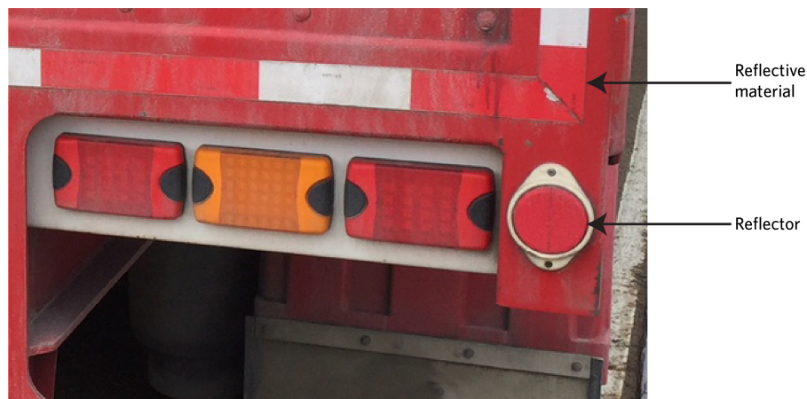
Figure 4-13-2. Reflector vs reflective material
