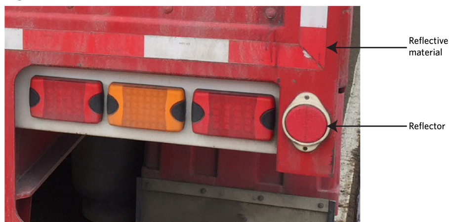
Figure 4-13-2. Reflector vs reflective material
