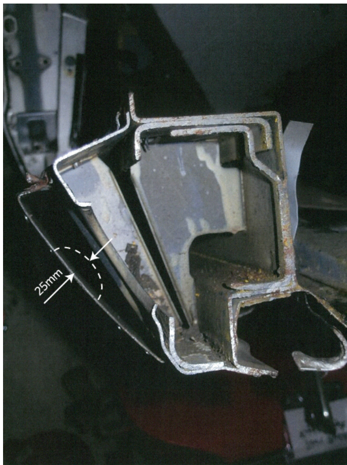
Figure 4-1-1. Outer sills cross section and rocker panels
