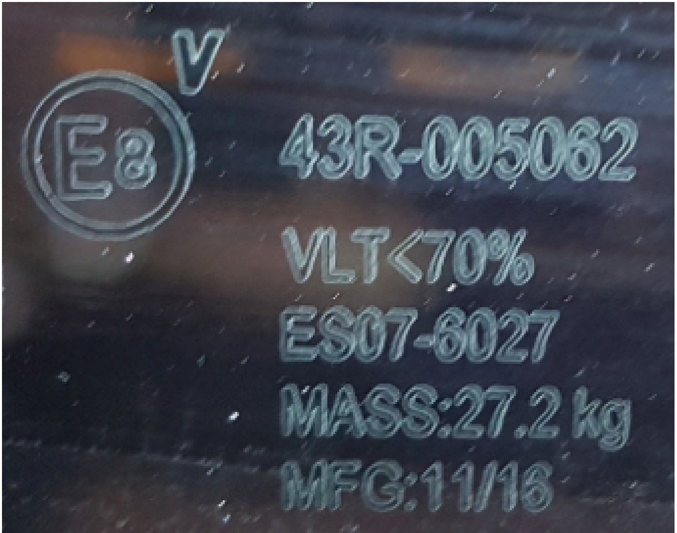
Figure 5-1-2. Typical laminated glazing markings (Note 1)
