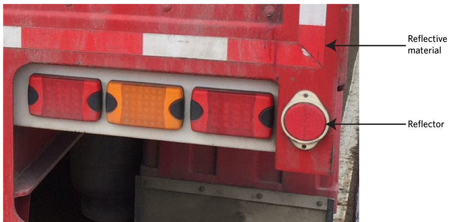
Figure 4-13-2. Reflector vs reflective material
