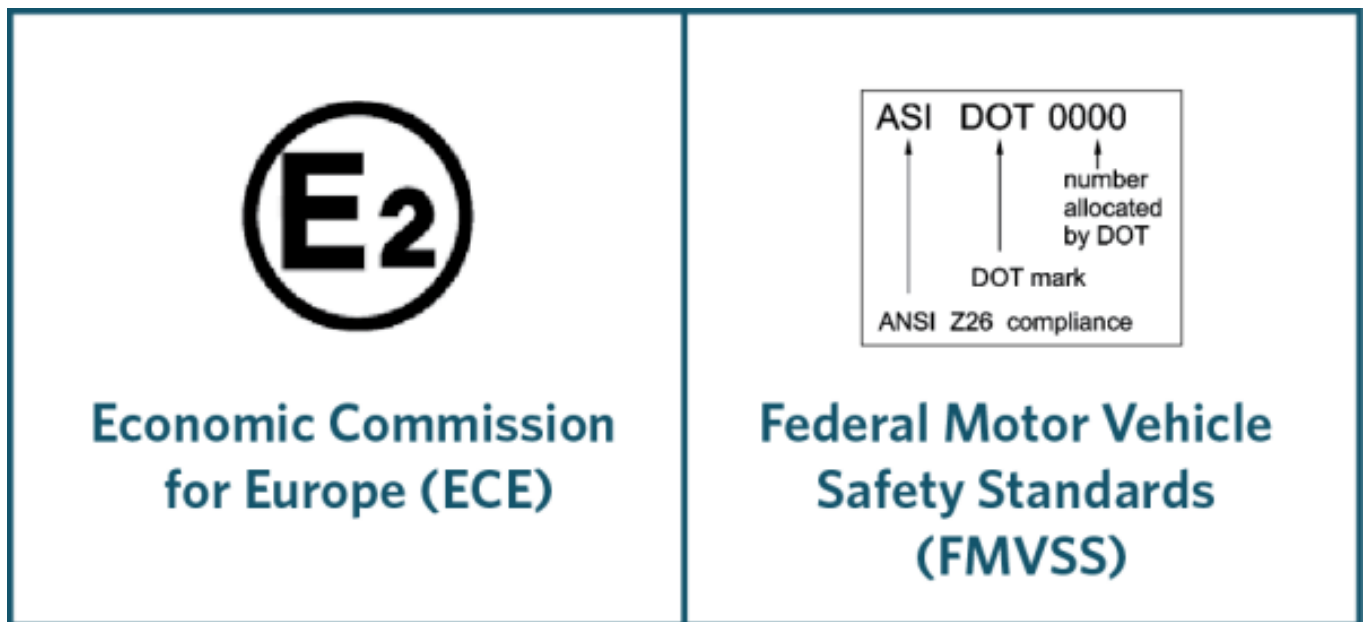
Figure 4-4-1. Approved daytime running lamp standard markings
