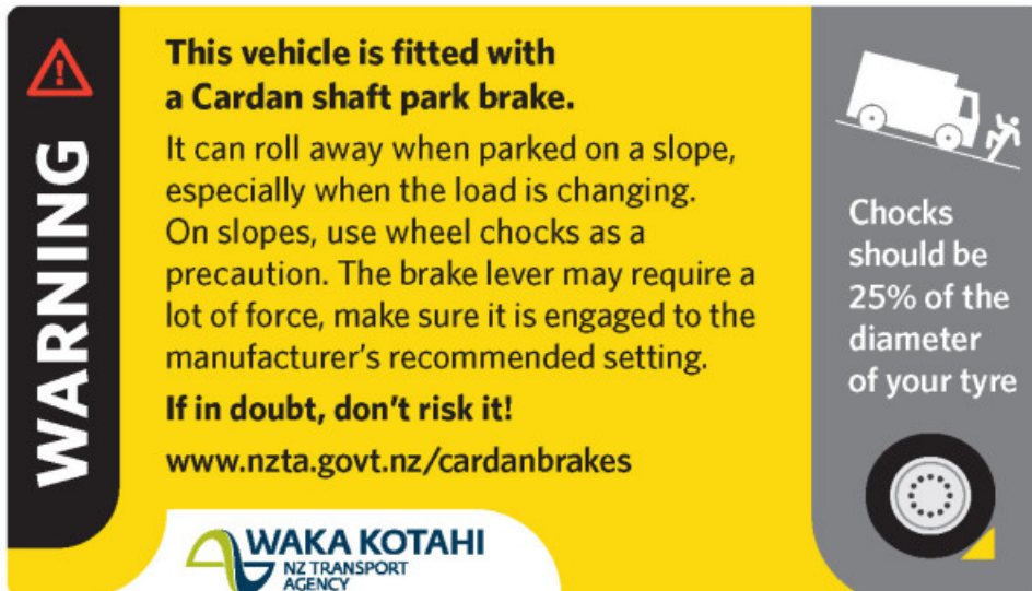
Figure 5-1-1. Cardan shaft park brake warning sticker
