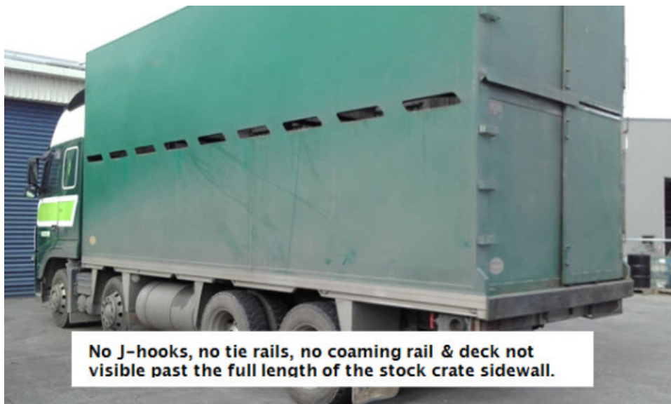
Figure 13-1-2. Monocoque stock transfer vehicle
