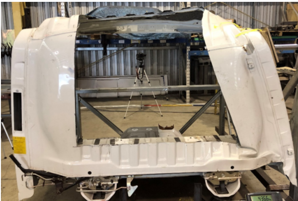
3-2 Modifications to the rear wall and roof where the structural rings of the cab have been removed
