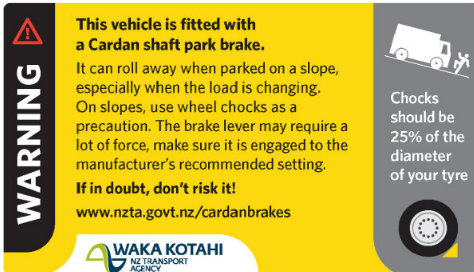
Figure 5-1-1. Cardan shaft park brake warning sticker
