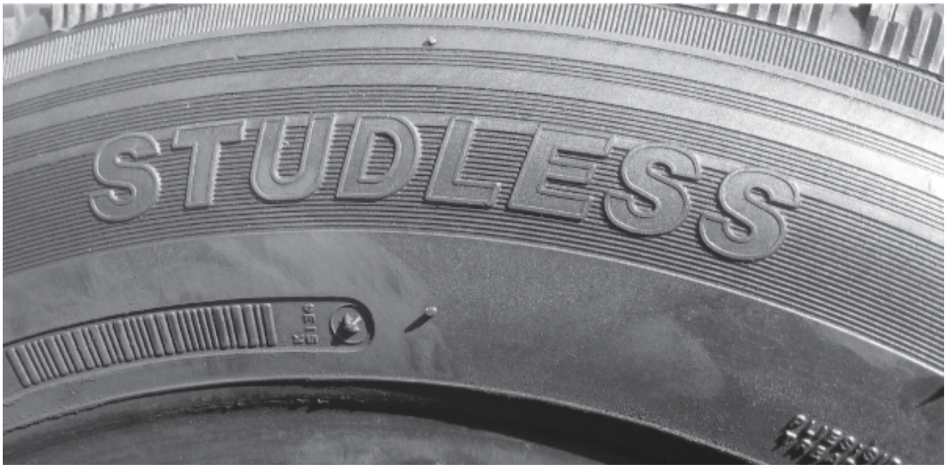
Example of 'Studless' on a tyre sidewall
