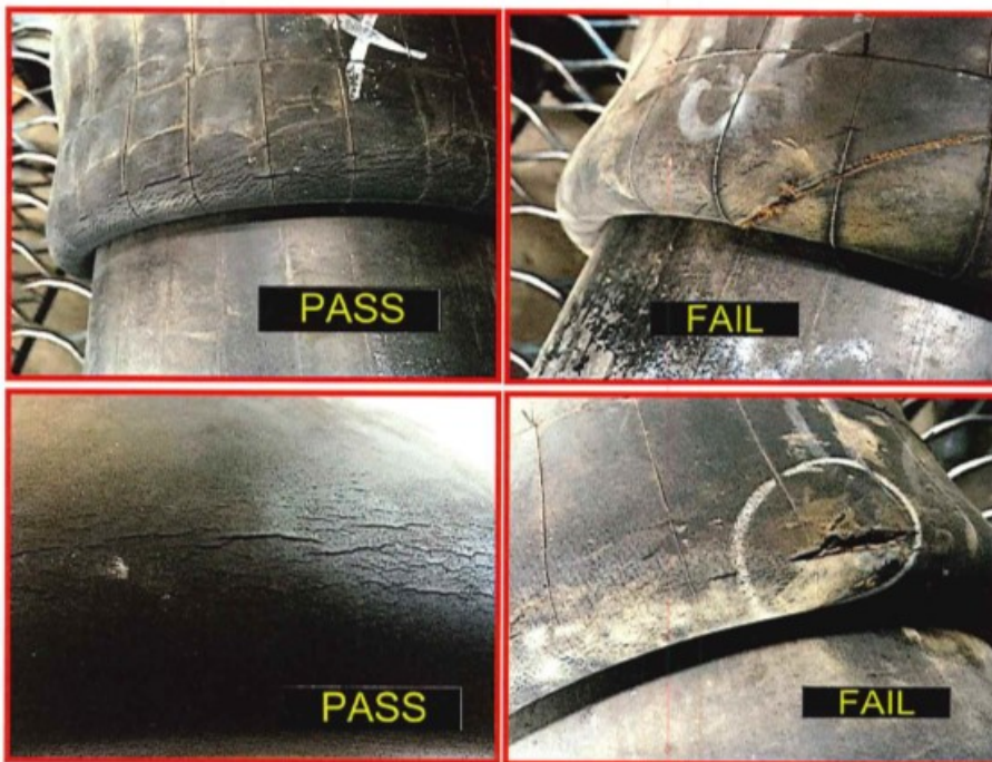
Figure 9-1-2. Sample air bag bellows images
