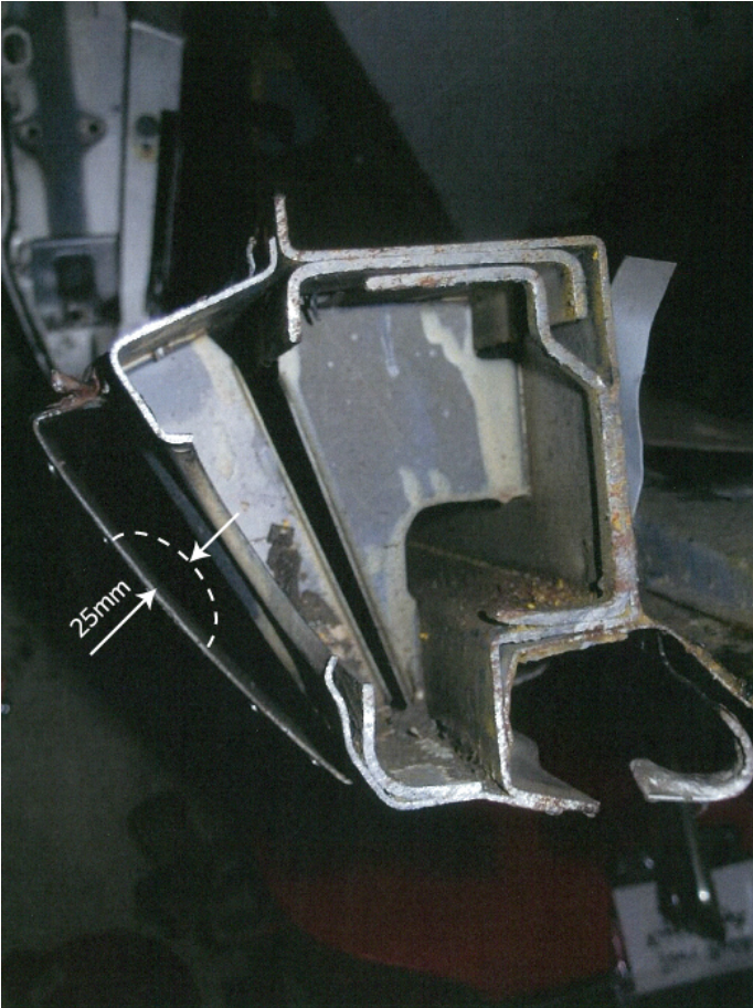
Figure 4-1-1. Outer sills cross section and rocker panels
