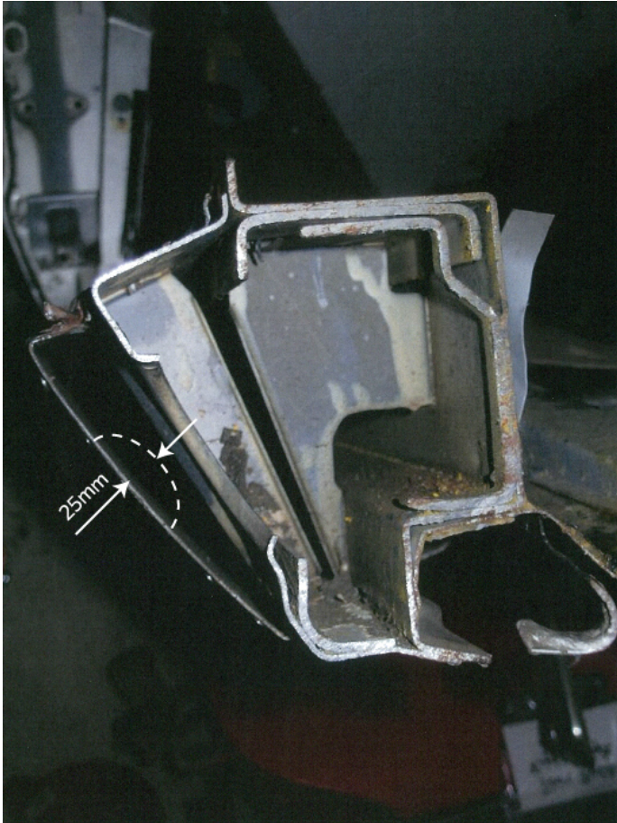
Figure 4-1-1. Outer sills cross section and rocker panels
