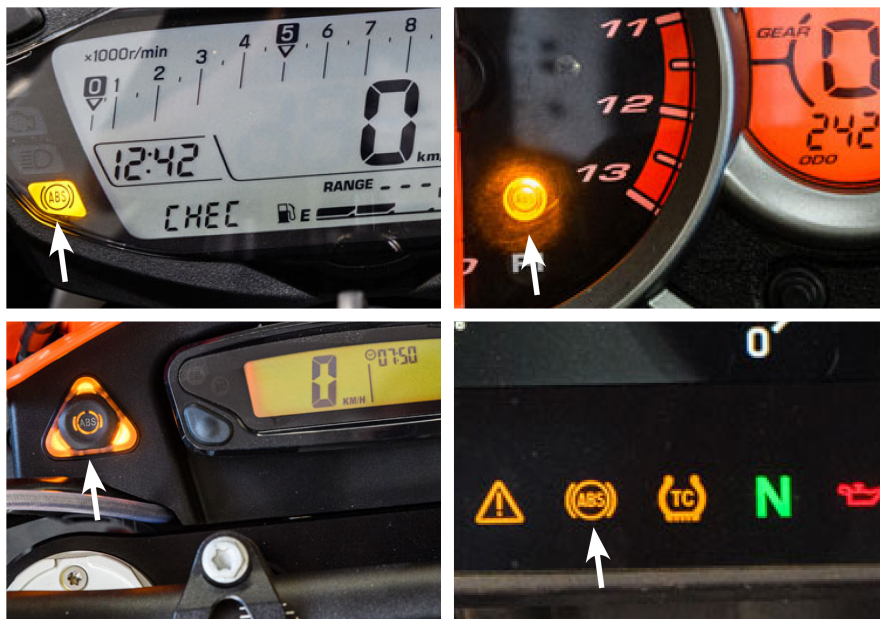
Figure 8-1-1. Examples of ABS warning light fault indication
