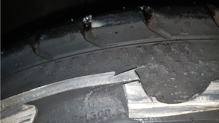
Example of tyre with information removed
