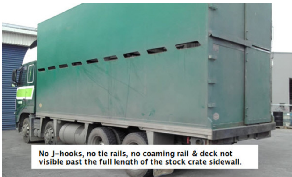
Figure 13-1-2. Monocoque stock transfer vehicle
