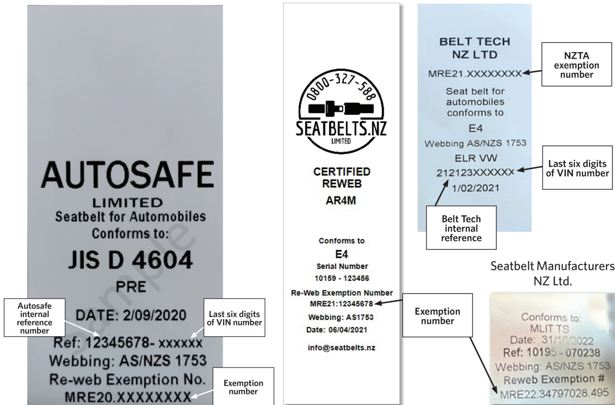
Figure 16-1-1. Sample Autosafe Ltd, Seatbelts NZ Ltd, Belt Tech NZ Ltd and Seatbelt Manufacturers NZ Ltd labels
