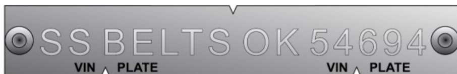
Figure 19-1-1 . Example of a single-sensitive seatbelt exemption plate
