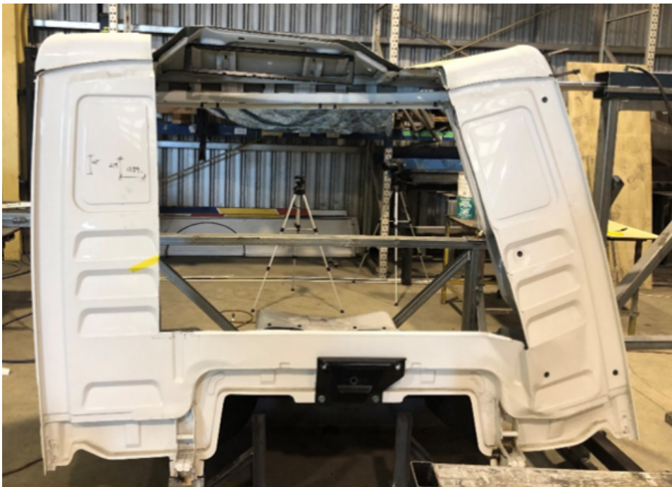
Figure 20-1-4. Modification to the rear wall and roof, Japanese (during testing)
