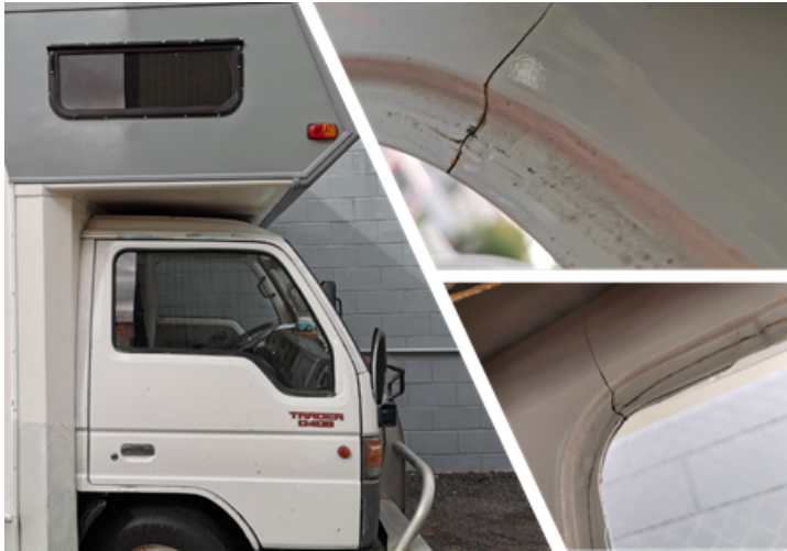
Figure 20-1-14. Cracks developing due to insufficient reinforcement after cab modifications
