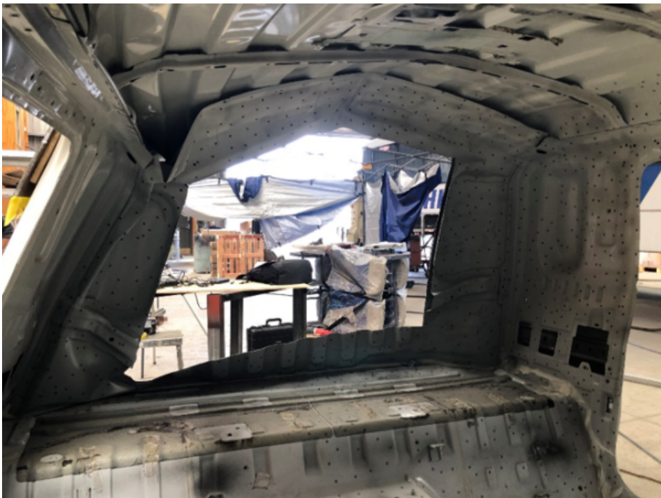
Figure 20-1-2. Modifications to the rear wall only, Japanese (after testing)
