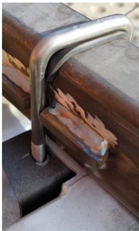
Figure 8-1-4. New front mount of the repaired Trailpro 8x4 and 8x5 trailers
