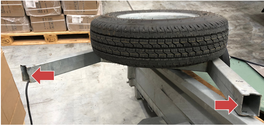
Figure 3-1-6. Trailpro plate showing repaired status
