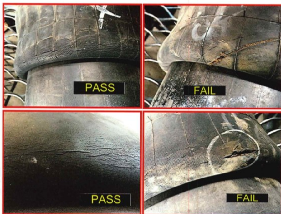
Figure 9-1-2. Sample air bag bellows images
